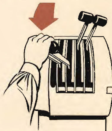
LOW BLOWER TO HIGH BLOWER
