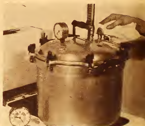
11. Fasten lid securely on canner. Let steam pour from open pet cock or weighted gage opening for at least 10 minutes. Then shut pet cock or put on weighted gage.
